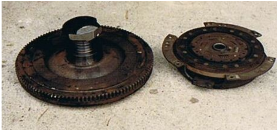
Flywheel and Clutch Assembly
