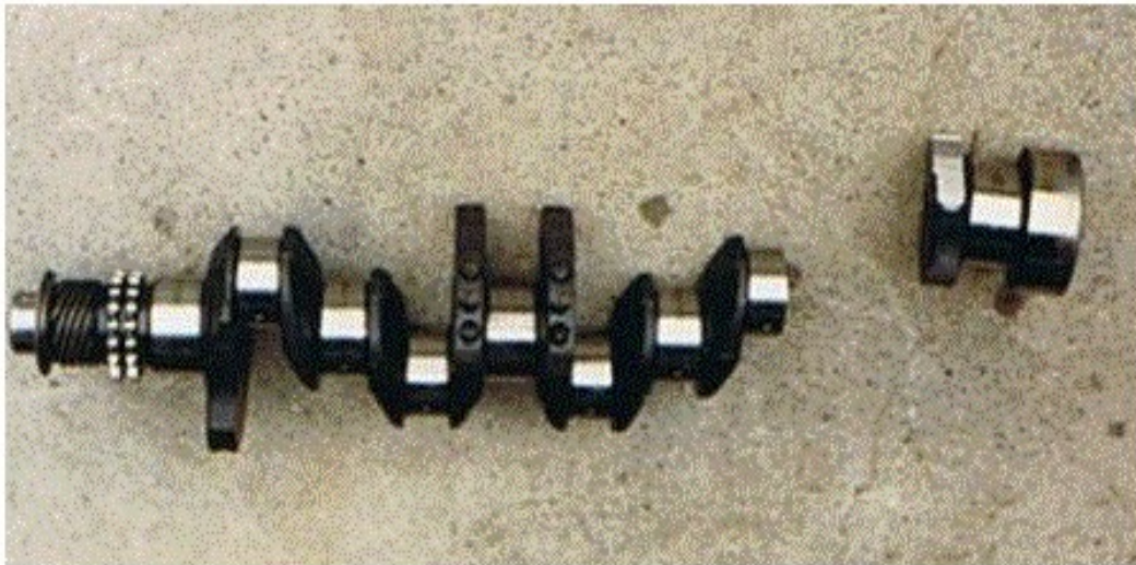
The Flywheel Flange is cut from the crank
