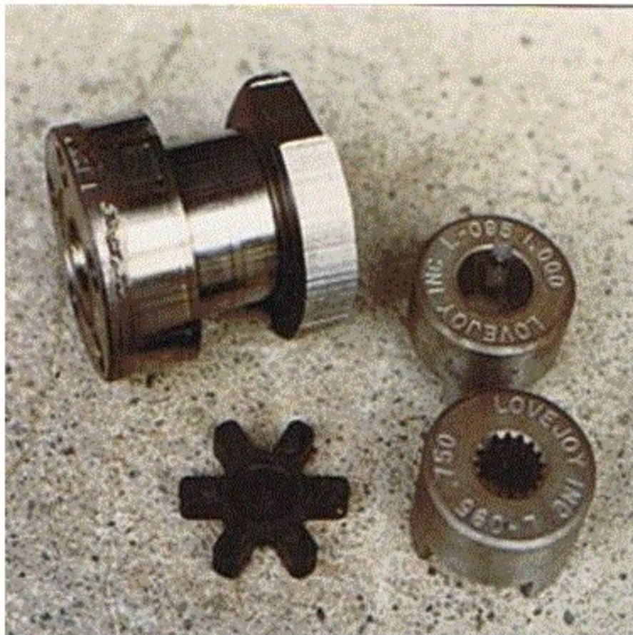
The Flex Coupler has three parts, spline on one side (lower) and Keyway on the other (upper).
