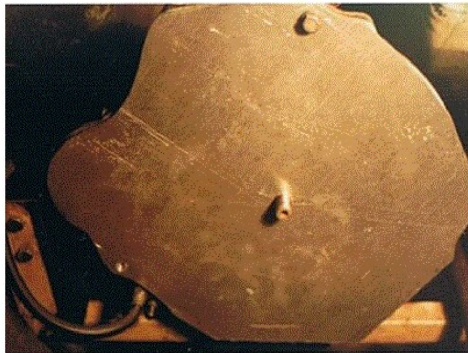
Trial fit of the Adaptor Plate
