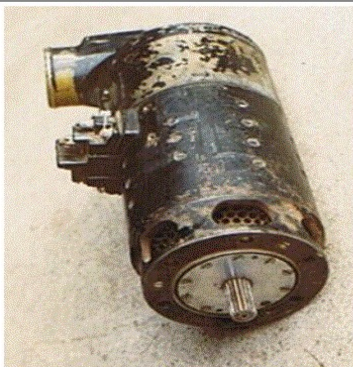
Bauer E-1604-1, aircraft Generator, 30V, 400 Amps, 4500-8000 RPM, Splined Drive shaft.
